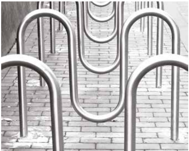
Camden 'M' stand Parks 2 bicycles and is a variation of the Sheffield stand and encourages locking the bicycle frame in two places.
