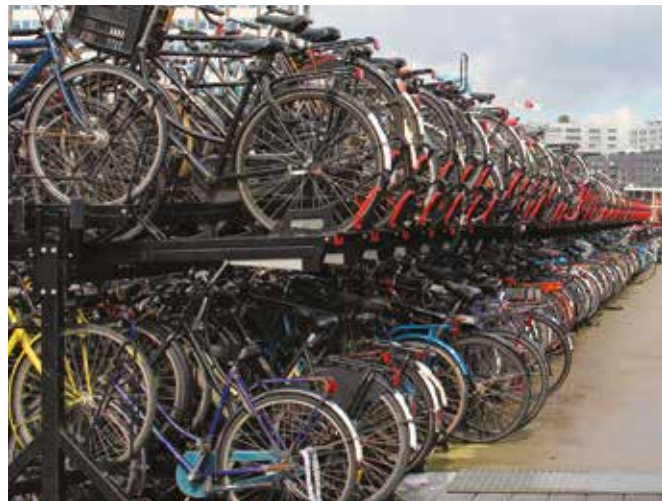
Two-tier stand Adds capacity by stacking bikes but should only be used for larger scale cycle parking and ideally be under cover (must meet criteria laid out in Section 4.2 of this document). Should not be used to provide 100% of cycle parking as they are not compatible with non-standard cycles and some users struggle to use them.
