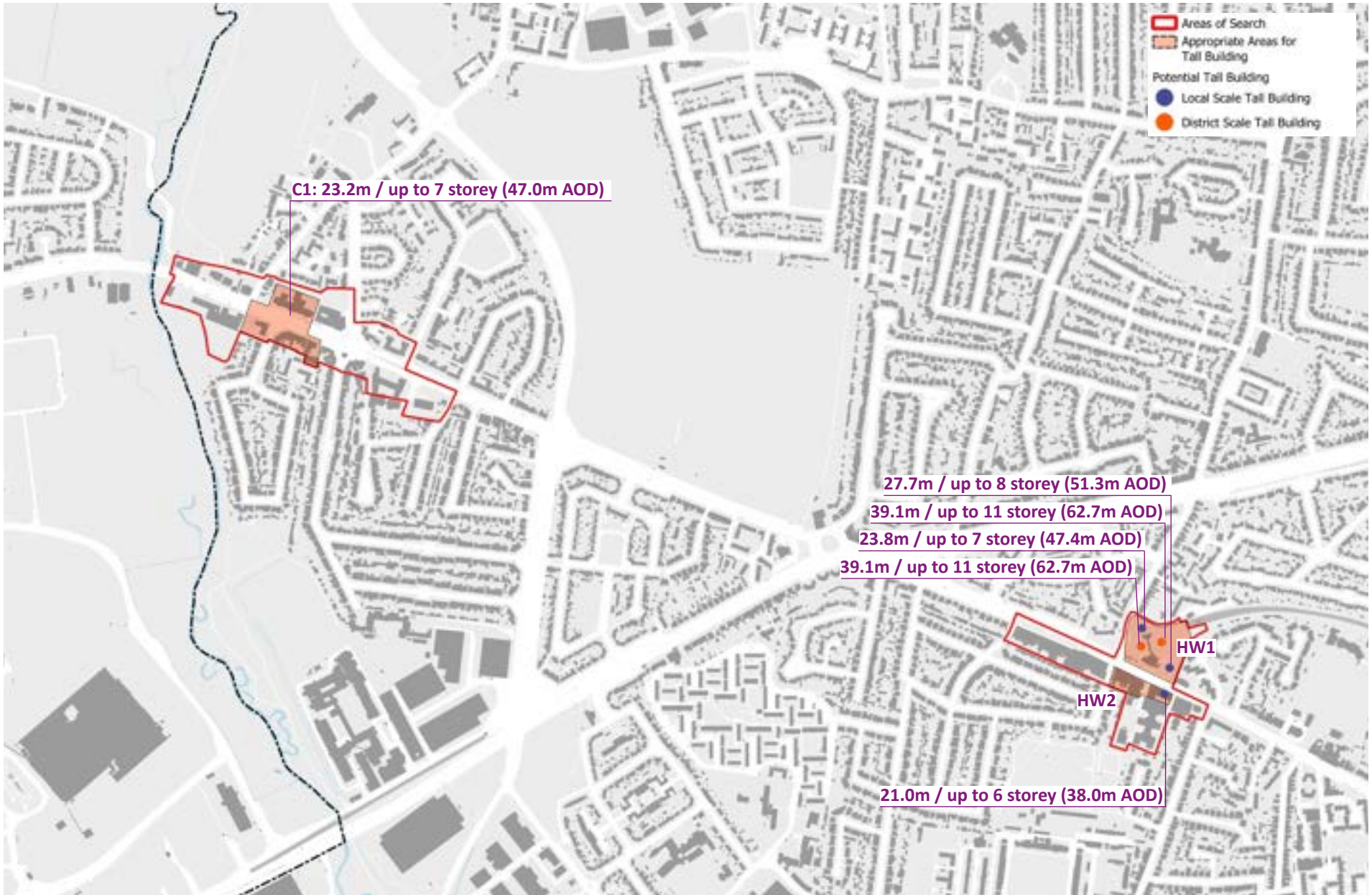
Figure 8.2: Bath Road Cranford and Hounslow West Area of Search - Tall Building Opportunities
