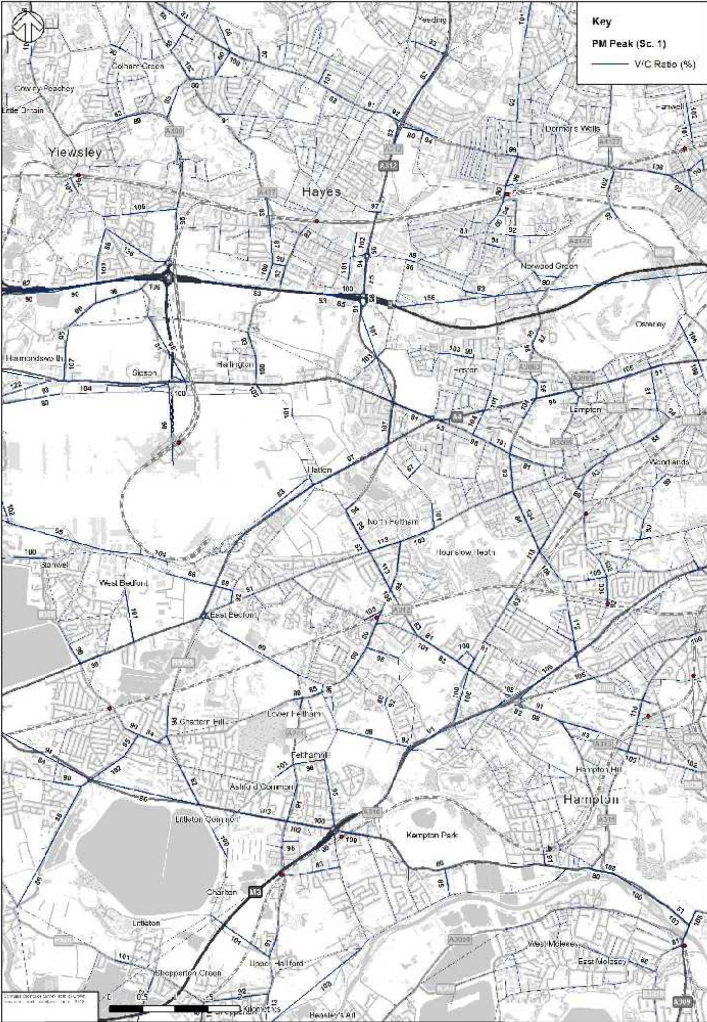
Fig. 2. Hampton road network, showing the V/C Ratio (%) for the PM Peak (Sc. 1) for the Hampton road network. The map is based on the Hampton road network data provided by the Hampton Council. The map is based on the Hampton road network data provided by the Hampton Council.
