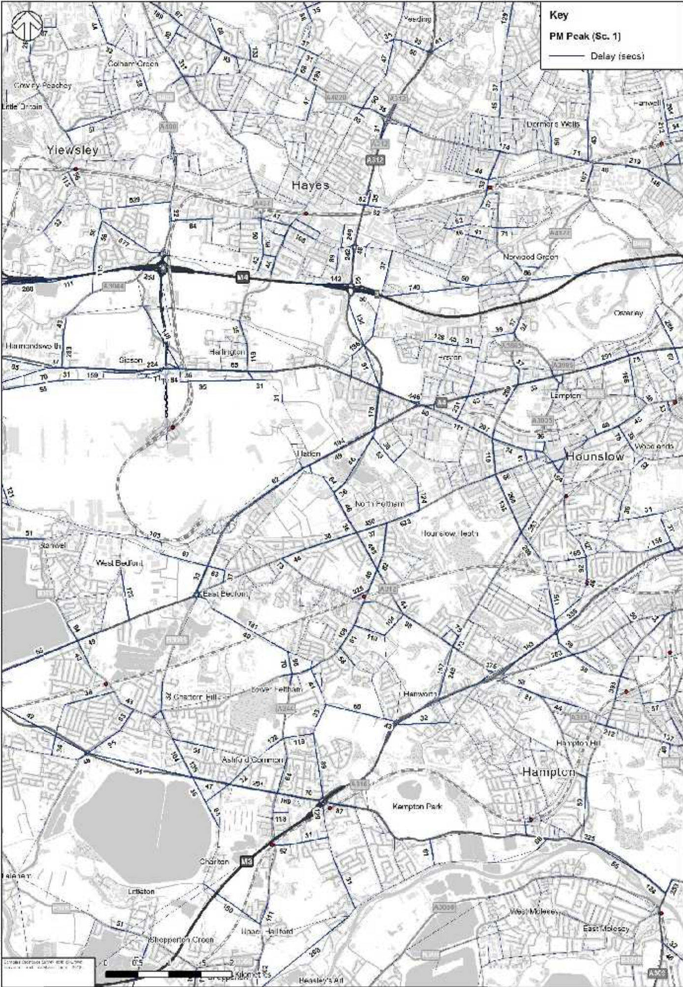
Fig. 2. Example of a typical road network showing the PM Peak traffic delay in seconds during the PM Peak (Scenario 1) in the Greater London area. The map shows the road network and the traffic delay in seconds during the PM Peak (Scenario 1) in the Greater London area. The map shows the road network and the traffic delay in seconds during the PM Peak (Scenario 1) in the Greater London area.
