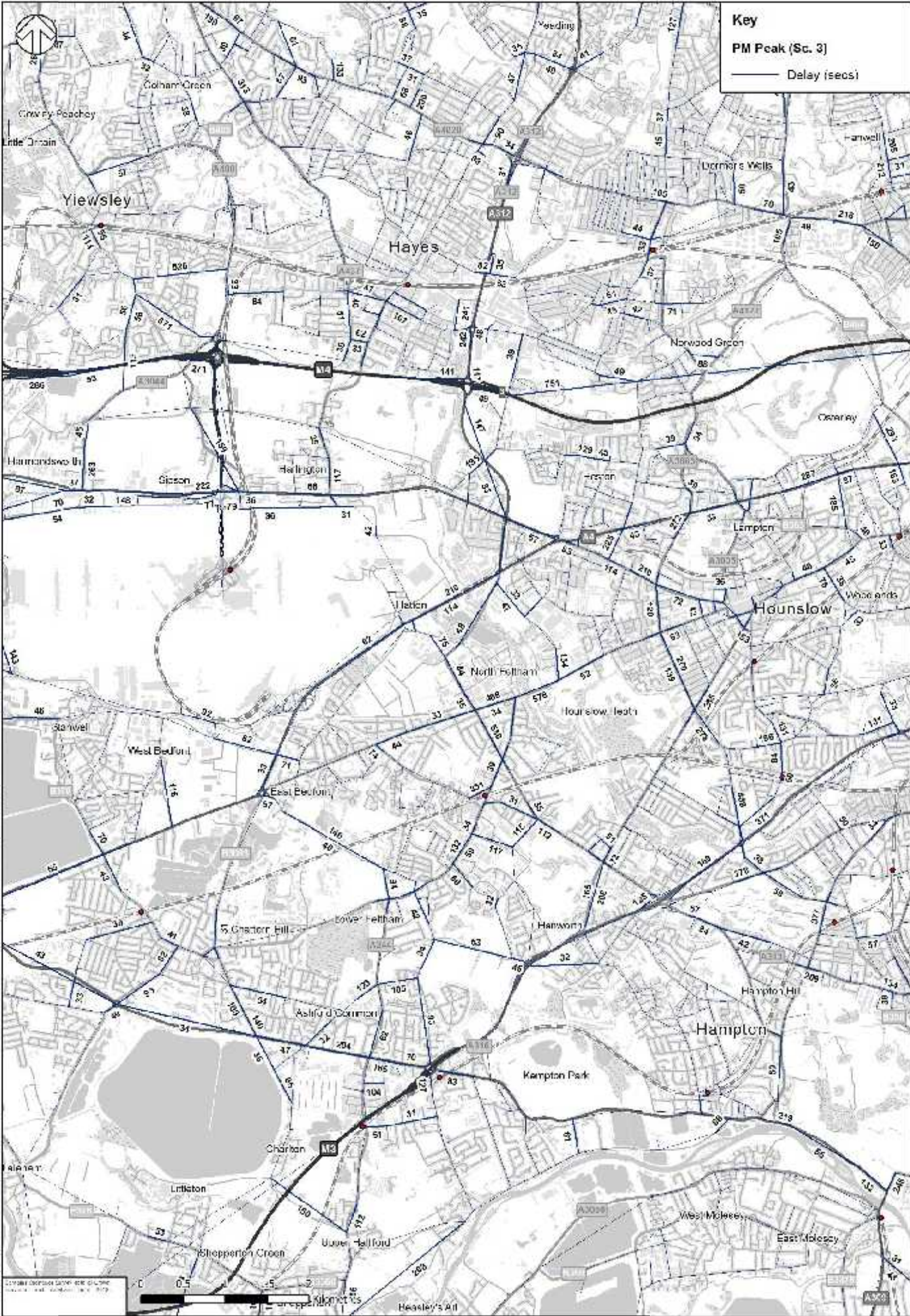
Fig. 2. Example of a typical delay map for the PM Peak (Scenario 3) in the London area. The map shows the delay in seconds for each road segment during the PM Peak (Scenario 3) in the London area. The map shows the delay in seconds for each road segment during the PM Peak (Scenario 3) in the London area.
