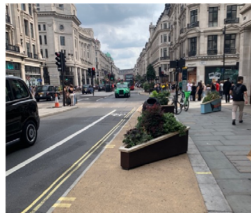
Fig B1.18 Street improvements on Regent Street have included pavement widening, cycle lane introduction and greening
