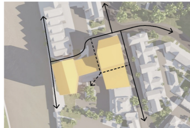
6 Public routes (solid) around the site and along the river should be retained and improved. Private pedestrian routes (dotted) should be introduced for access to the courtyard.
