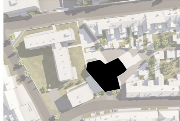
2 The footprint of the backland development should respond to the particular geometry of the site.
