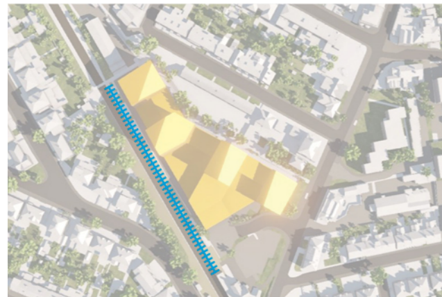
9 Retain a minimum distance (determined by the rail operator) for the safeguarding zone. The boundary between the development and the railway platform should be improved and made more solid to screen new homes from train-related activity. Buffers such as planted walls or art murals may create a better defined and more attractive separation.
