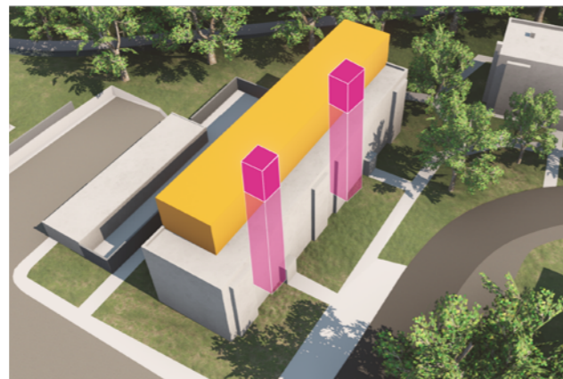
6 Access to the additional storey is achieved through extending the existing circulation.
