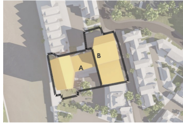
1 A phased demolition would allow one section of the building (B) to remain in use while the first phase of the new development (A) is under construction.
