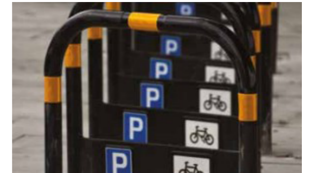
Fig A2.18 Sheffield parking stands - Parks two bikes, and the most cost effective cycle parking solution. Supports different types of cycles. Can lock both wheels © West London Cycle Parking Guidance, 2017.
