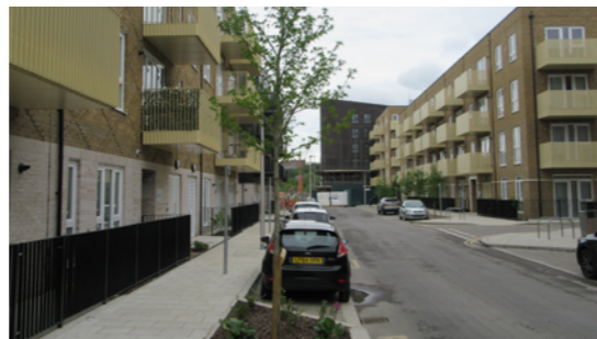
Fig A2.23 Off - street car parking with strong defensible boundary to the street, Rochester Riverside. © Allies and Morrison
