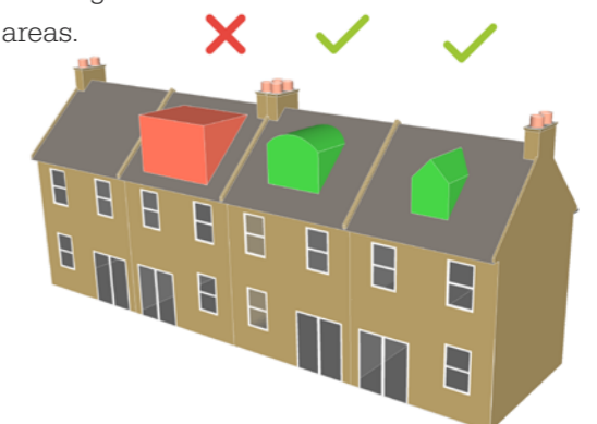
Fig A5.24 Dormer window extensions should be of modest size and not dominate the roof.
