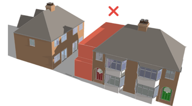
Fig A5.10 Side extensions will not be permitted where the rear windows of houses face the side wall of the house in question
