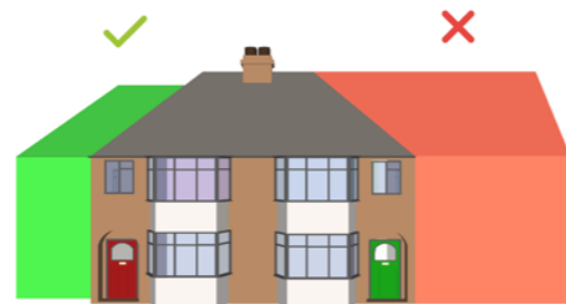
Fig A5.8 Side extensions should normally be set back at least 1m from the original front house wall
