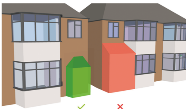
Fig A5.16 Front porches should be small and minor to the appearance of the house
