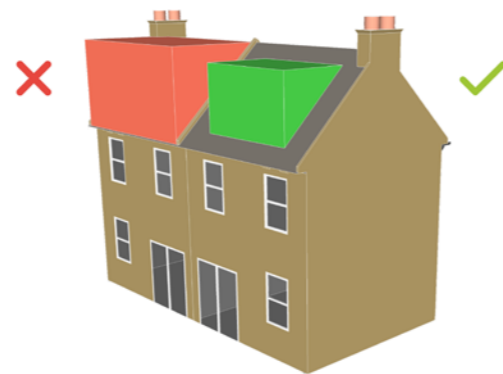
Fig A5.19 Roof extensions should be set in the centre of the roof face
