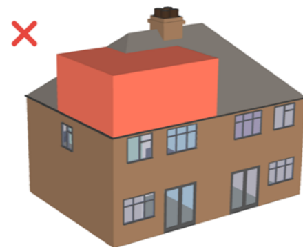
Fig A5.21 Extensions should not extend to the full house width and not wrap around two planes of the roof
