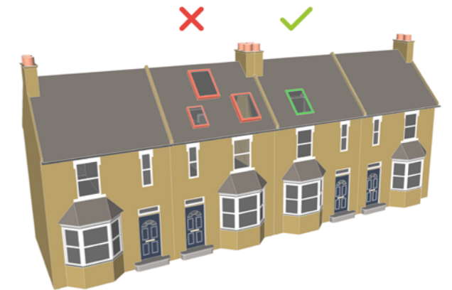
Fig A5.23 Roof lights should respect the size and position of windows in the main house
