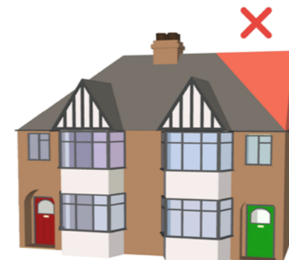
Fig A5.18 Converting a sloped hip-end roof flat gable-end roof would unbalance the appearance of the house
