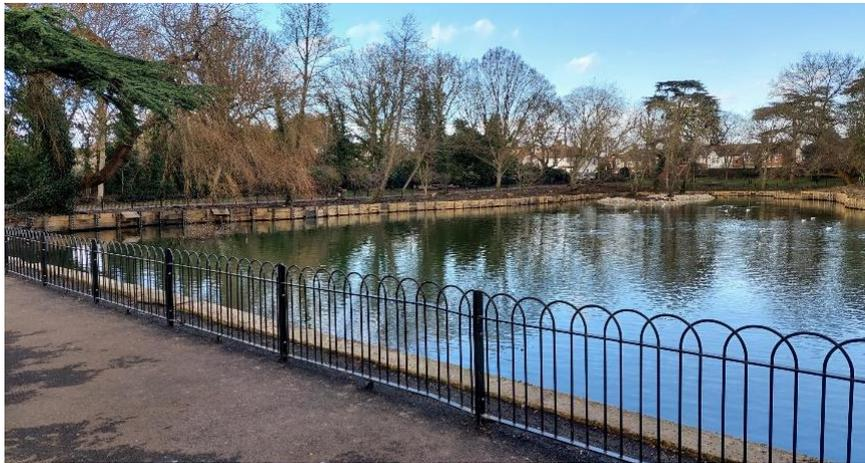
*Figure 18 Restored Lake with new fencing and observation platform, wood revetments to retain the 700 tonnes of excavated silt.*
