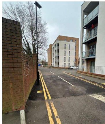
There is a concern that this lighting column may not be clearly visible to drivers, particularly if the lighting column is not working during the hours of darkness. This may result in the lighting column being struck by a passing vehicle causing vehicle damage and/or damage to the lamp column, with potential injury to other road users travelling along Manor Lane.
