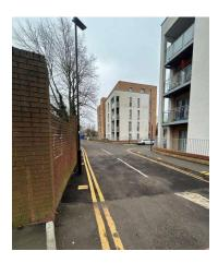
There is a concern that this lighting column may not be clearly visible to drivers, particularly if the lighting column is not working during the hours of darkness. This may result in the lighting column being struck by a passing vehicle causing vehicle damage and/or damage to the lamp column, with potential injury to other road users travelling along Manor Lane.
